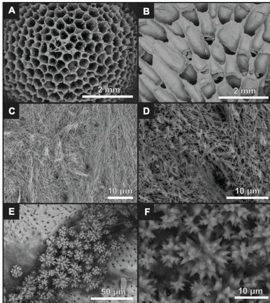
**Fig. 3** Scanning electron micrograph images of sclerosponges. A well-preserved pristine calcite skeleton is visible. **A** and **B** Macrostructural organization of high-Mg calcite skeleton with vertical calicles subdivided by horizontal tabulae. **C** and **D** Lamellar microstructure of high-Mg calcite skeleton, the secondary structure of the tabulae and coatings of the tubes, randomly oriented single crystals. **E** and **F** Spicular skeleton and spiraster microscleres
