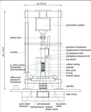
**Fig. 3** Schematic sketch of the triaxial deformation apparatus used for compressional testing in the laboratory experiments
