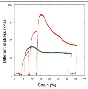
**Fig. 4** Differential stress/strain curves for single compression test (dark green) and pressure stepping test (red) from sample C0001E6H-1
