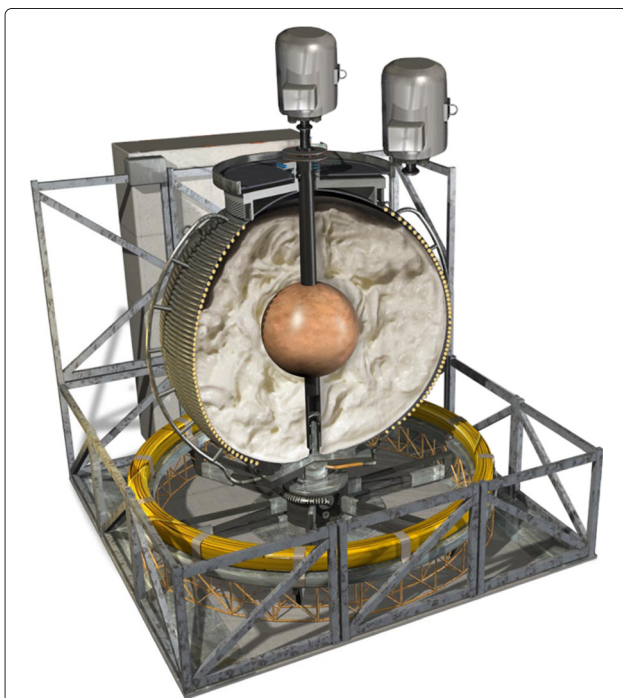
Fig. 2 Rendering of the 3 m experiment. The inner sphere and the outer spherical shell can be driven independently by their two respective motors (top). Liquid sodium serves as the working fluid for hydromagnetic experiments
