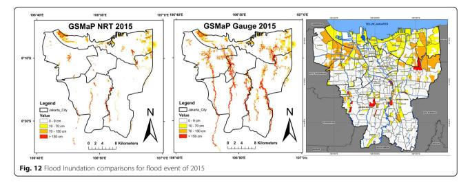
From these results, we concluded that the GSMaP Gauge data could be used to reproduce previous flood inundation events in Jakarta. However, it is challenging to use GSMaP NRT data as the input in a real-time flood-forecasting system owing to its low accuracy.
