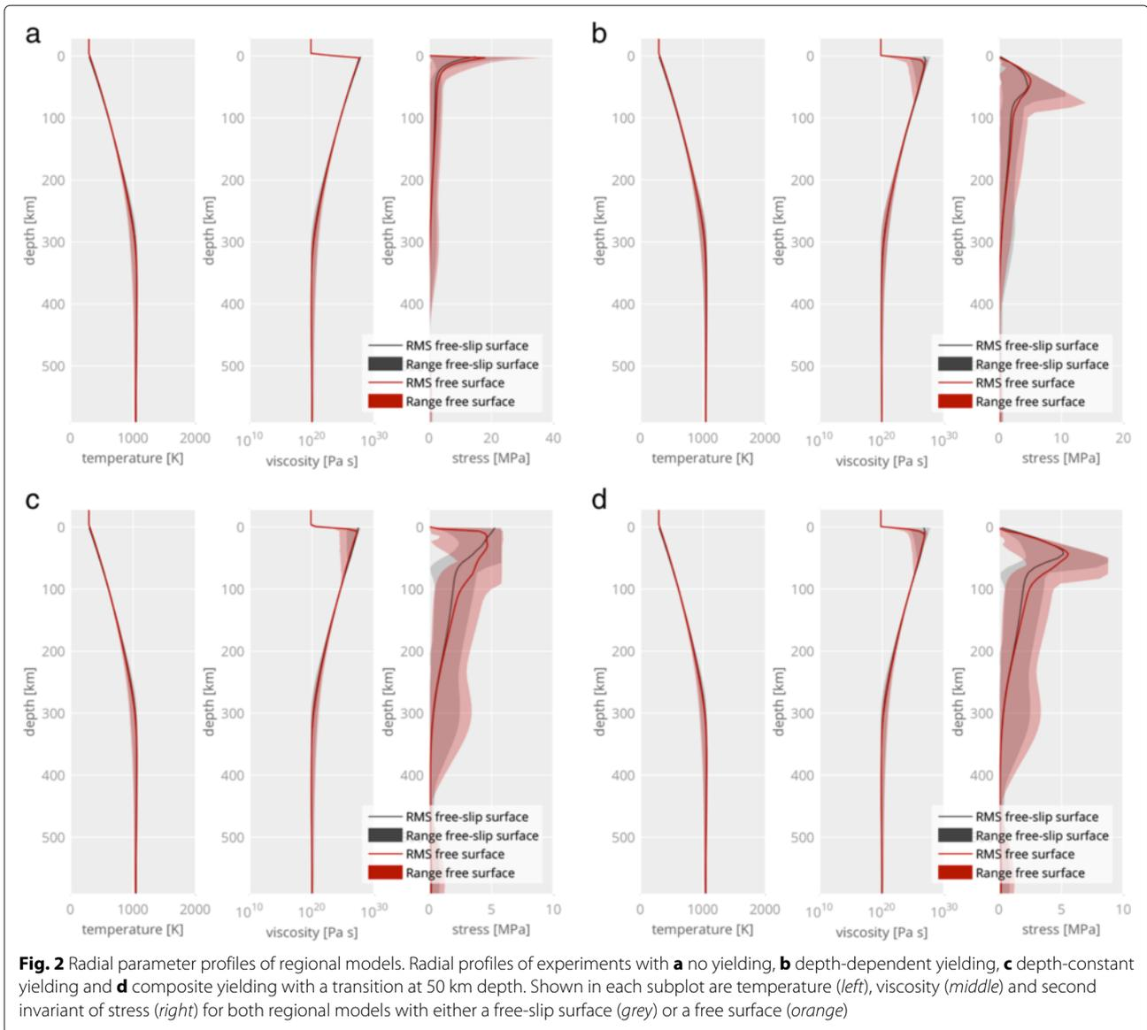
The maximum ductile yield stress that still allows subduction to occur is  $\sigma_{y,\text{const}} = 0.0005$  (7.3 MPa) and  $\sigma_{y,\text{const}} = 0.00065$  (9.5 MPa) for the free-slip and the free surface model, respectively. Limiting the strength of the lithosphere at shallow depth therefore allows for a 64 % stronger lower part that still entirely yields and subsequently subducts.
