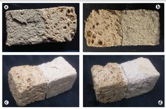
**Fig. 10** Cracks observed at and parallel to stone/mortar interface due to frost damage. **a** T and coarse porous limestone. **b** Coarse porous limestone and T50. **c** Coarse porous limestone and K. **d** Coarse porous limestone and K50
